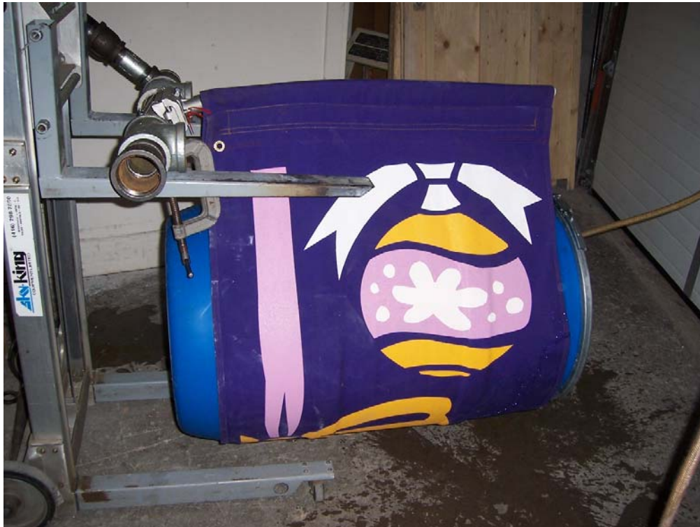
Assembly with load (blue barrel filled with water wrapped by the decorated banner).
